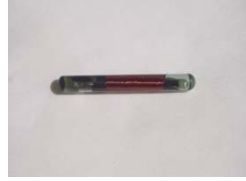
Figure 8 : Transpondeur TIRIS (Texas Instrument Radio Identification System)
