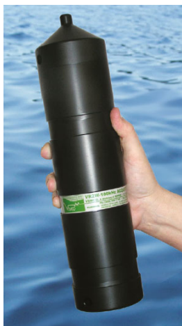
Figure 27 : Hydrophone VR2W – 180 kHz
